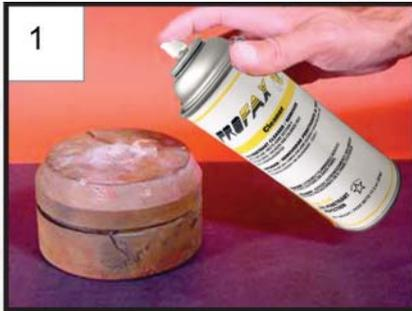
Use Profax cleaner to remove dirt, oil, grease, anti-spatter from surface area.
