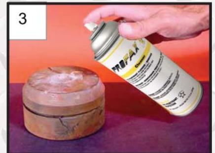
Remove penetrant from surface area (do not flush) using Profax cleaner.
