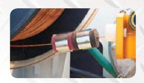
Weldaid Lube - Matic products are engineered to clean and lubricate welding wire, improve feedability, reduce weld spatter and increase tip and liner life.
