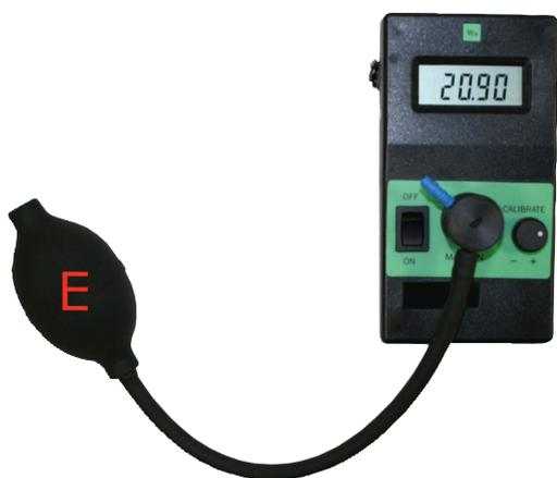
6. Connect the hose fitted to the aspirator bulb (E) to one port of the flow adaptor.
