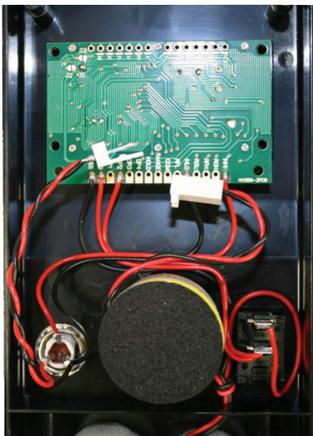
4. The sensor (I) is wired to the circuit board. Wires are connected to the sensor by a pin connector which can be disconnected by lifting the locking latch on the connector outwards. The connector can be lifted off the connector housing which is located on the circuit board.
