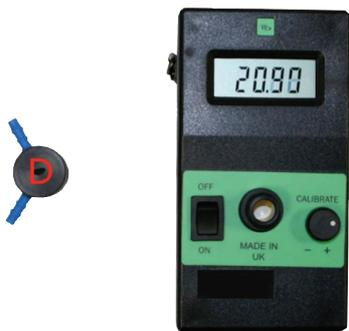
5. Connect the flow adaptor (D) to the sensor outlet of the Weld Gas Analyser.
