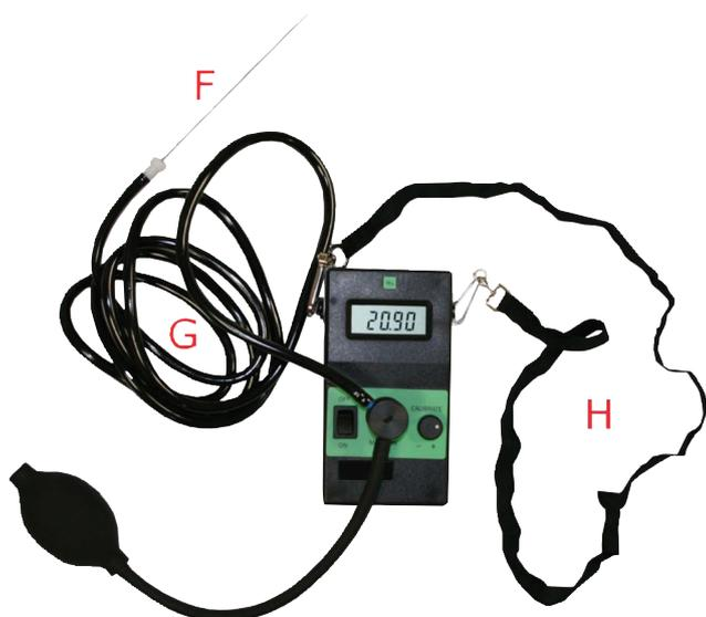
7. Connect the steel sampling probe (F) to one end of the rubber hose (G) and connect the other end of the hose to remaining port of the flow adaptor.
