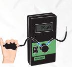
• Squeeze aspirator bulb to take a sample of the weld purge area gas, you will notice that the dial on the self calibrating unit will change according to the oxygen level inside the purge area.
