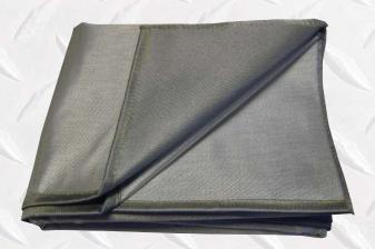
Kronos is a Thermo E Glass fabric with a specially formulated grey fire retardant PU coating on one side with aluminium pigments to increase the antislip properties & resistance to fraying. The maximum application temperature is 550°C (peak up to 600°C).
