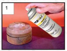
Use Profax cleaner to remove dirt, oil, grease, anti-spatter from surface area.
