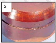
Apply Profax penetrant around area being inspected.
