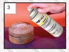
Remove penetrant from surface area (do not flush) using Profax cleaner.
