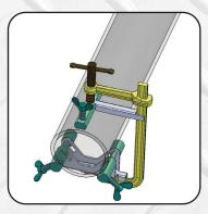
Turn three adjustment screws to preset.
