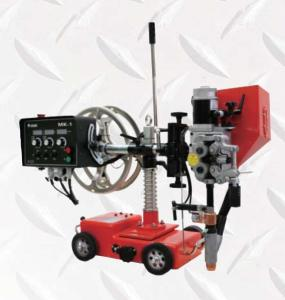
Suitable for all medium steel plates butt joint welding, lap joint welding, angle joint welding and overlaying welding. Applicable to all kinds of steel structure, stainless steel, heat resistant steel and nickel base alloy steel; can be used as overlaying welding equipment and is equipped with carbon arc gouging functions. Wide application in ship building, boiler, wind power industry, pipeline, weight-lifting equipment and pressure vessels.
