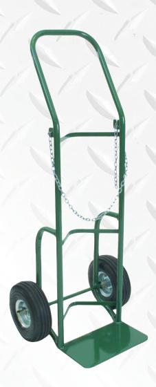
Popular cylinder truck can be used for gas cylinders up to 12" (30 cm) in diameter or for hauling boxes on the 7 x 14" (17.8 x 35.6 cm) base plate. Load capacity rated at 500 lb (225 Kg).
